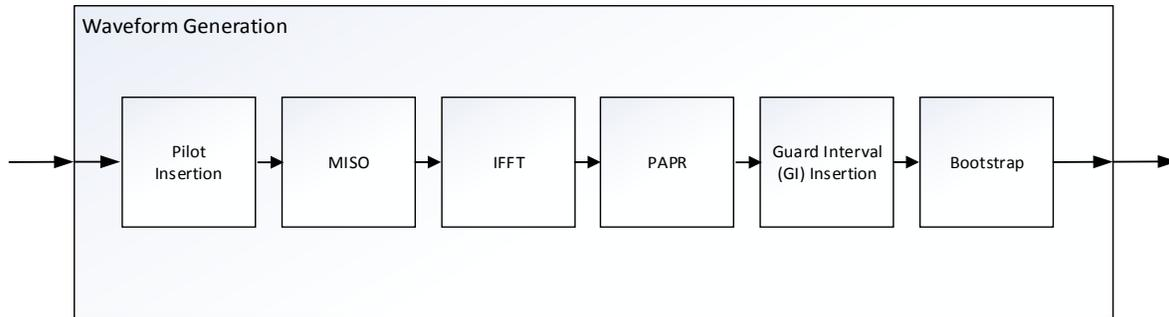
**Figure 21: Block diagram of waveform generation**
