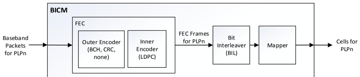
**Figure 15: Block diagram of BICM**
