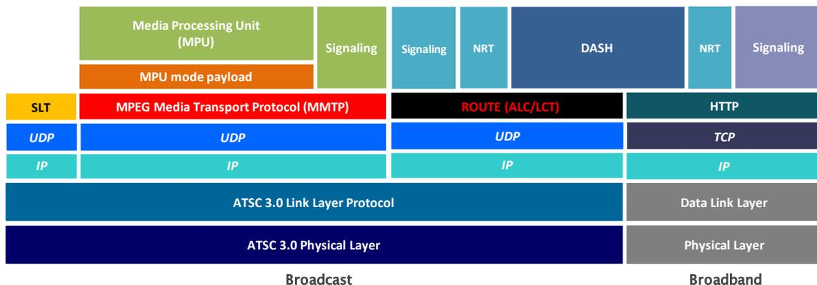
**Figure 7: ATSC 3.0 receiver protocol stack**
