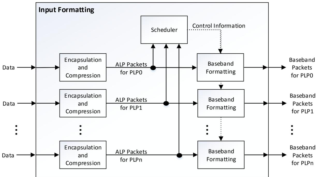
**Figure 13: Block diagram of input formatting**
