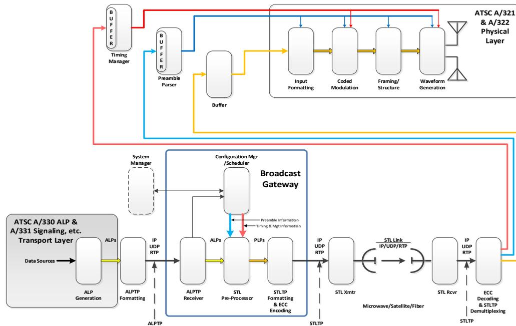
**Figure 8: High Level Overview of System Configuration**
