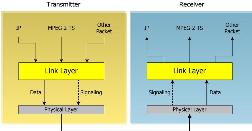
**Figure 5: ATSC 3.0 link layer logical diagram**
