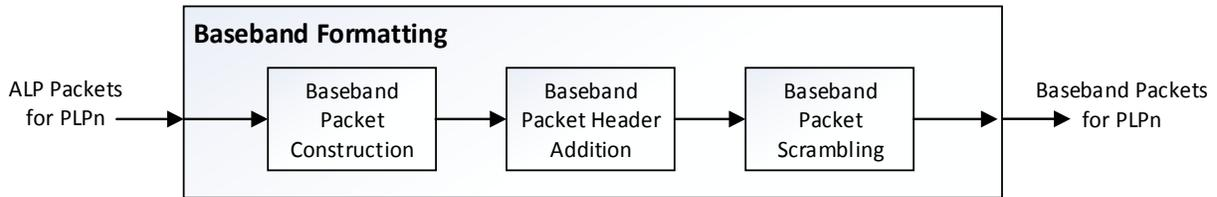
**Figure 14: Block diagram of baseband formatting**
