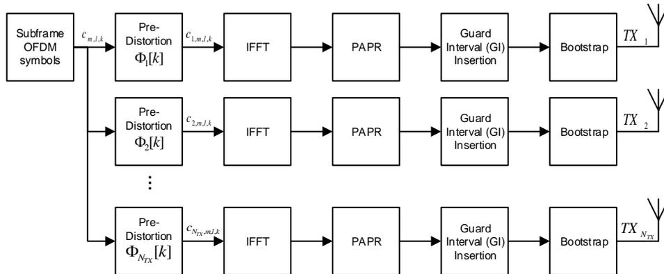
**Figure 22: Block diagram showing example MISO transmission**
