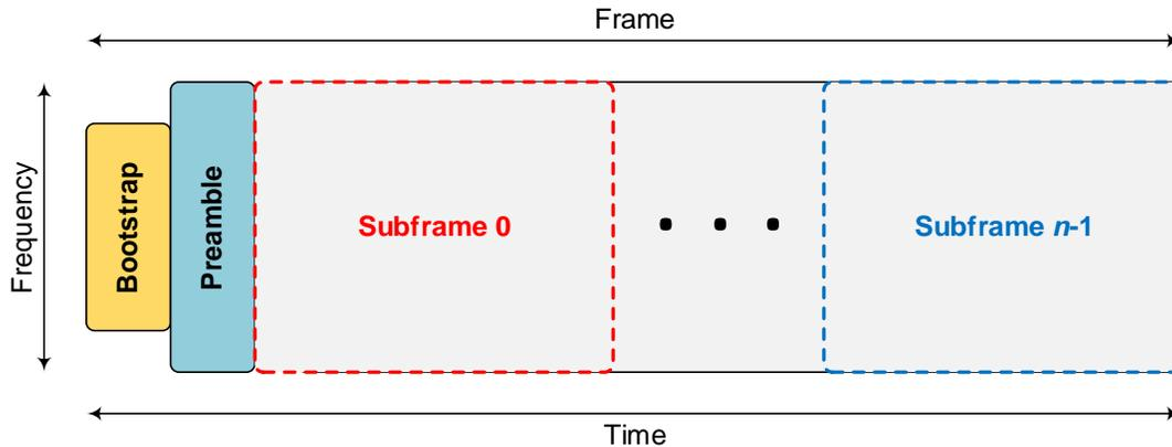
**Figure 11: Frame structure**
