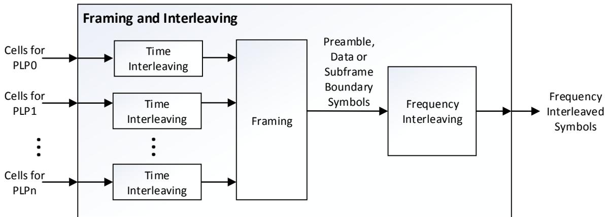
**Figure 20: Block diagram of framing and interleaving**
