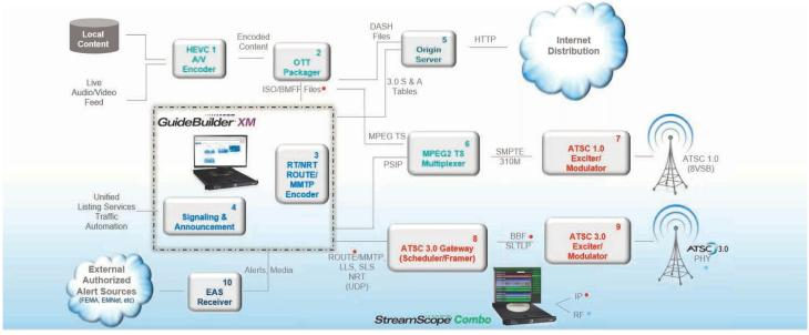
The StreamScope Combo analyzer validates, monitors, and troubleshoots transport streams throughout ATSC 1.0 and ATSC 3.0 broadcast chains.
